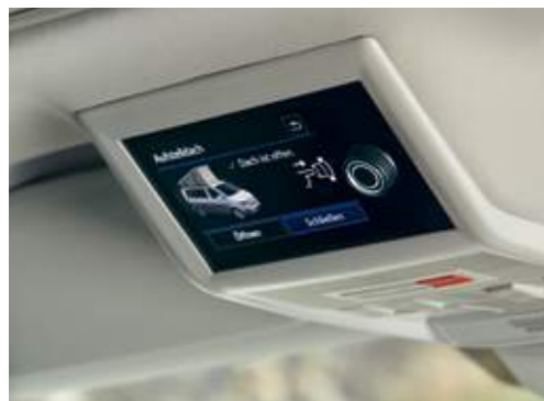
Control of the electro-hydraulic elevating roof 1)
