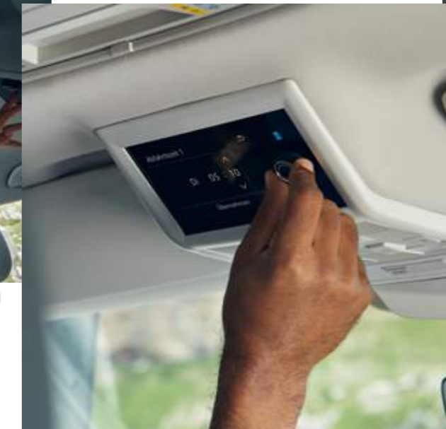
The auxiliary heater can be set to continuous operation for the night on the new Camper control unit.
